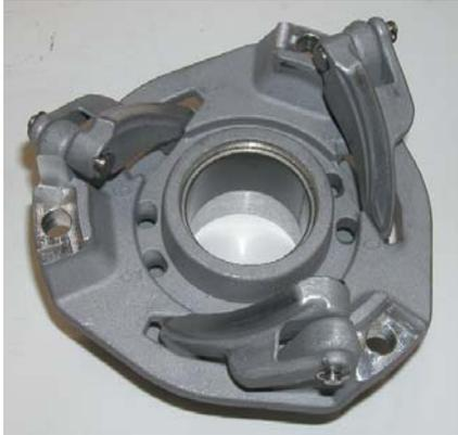
The premise is simple; provide a quick-adjust method of varying the angle of the helix ramps. Instead of having to remove and disassemble the secondary clutch, now you can adjust the helix angles with a simple twist of your wrist. It is so simple and effective, why doesn't every machine have one?
